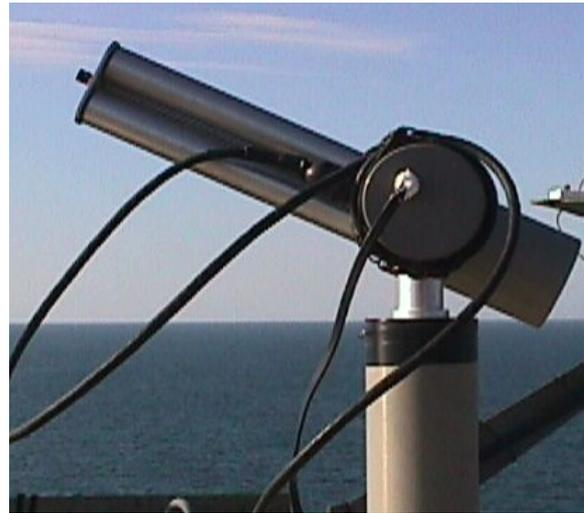
Figure 2. Sun Photometer AERONET NASA
