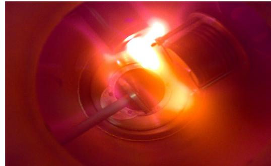
Fig.2 Close-up on the InN thin film deposition
