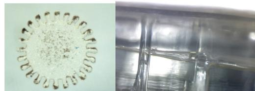
a.) b) Pic.5 a,b) The results of cutting a photovoltaic cell point by point with a circular mask and a slot mask c) wheel made directly with the mask
