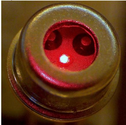
Figure 1. Picture of a red (670 nm) single mode VCSEL.
