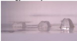
Pic.2 Some result of total pulse number influence for angle between channel wall and entrance surface. The tests were made for a fixed fluency of  $2\text{J}/\text{cm}^2$ , 3Hz and a total number of pulses between 300 and 550.
